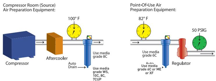
Any compressor with after-cooler, 2-stage coalescing. Air intended for use with lubricated control valves, cylinders, parts blow-down, etc.
