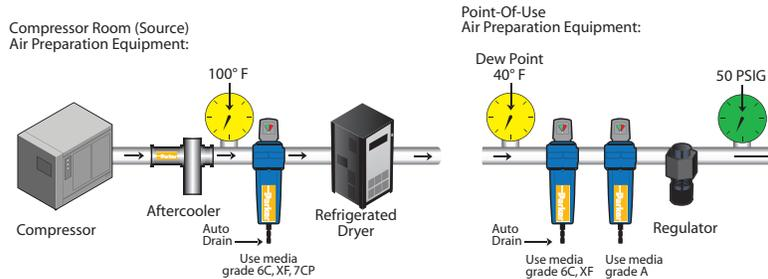
Any compressor with after-cooler, 2-stage coalescing, refrigerated dryer and carbon absorber. Air intended for use as industrial breathing air and decompression chambers. CAUTION: Always use high temperature synthetic lubricants and monitor (alarm for carbon monoxide concentrations). This system will not eliminate toxic gases!
