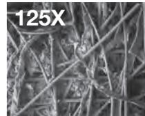
Stage 2 adsorbers polish the air stream of final trace amounts of hydrocarbon vapors with an efficiency of 99%+.
