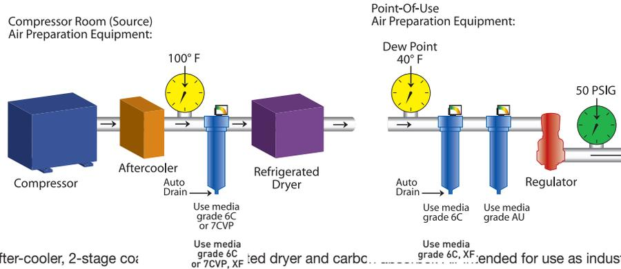
Any compressor with after-cooler, 2-stage compressed air system with a carbon canister and a refrigerated dryer and carbon canister. Air intended for use as industrial breathing air and decompression chambers.
