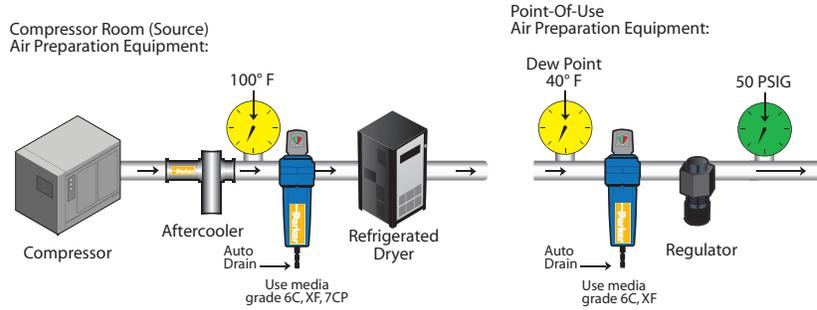
Any compressor with after-cooler, 2-stage coalescing and refrigerated dryer. Air intended for use with air gauging, air conveyors, spray-painting, food processing, instrumentation, blow molding, cosmetics, film processing, bottling, pharmaceuticals, dairy, breweries, medical, robotics and close tolerance valves.
