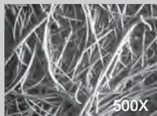
Grade 6 filter elements are used when “total removal of liquid aerosols and suspended fines” is required. Because of its overall performance characteristics, this grade is most often recommended below 500 PSIG.
