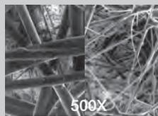
Grade 7CVP filter elements are made with two layers. The inner layer (left) effectively traps dirt particles, protecting and extending the life of the outer layer. The coalescing outer layer (right) consists of a dense matrix of glass fibers, providing highly efficient aerosol removal.
