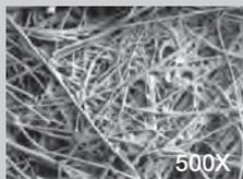
Grade 4 filter elements are very high efficiency coalescers; for elevated pressures or lighter weight gases. Recommended when system pressure exceeds 500 PSIG.
