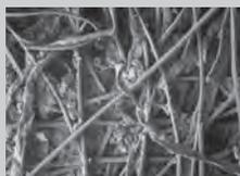
Three micron pleated cellulose filters are used for particulate interception where very high dirt holding capacity and a relatively fine pore structure are required.
