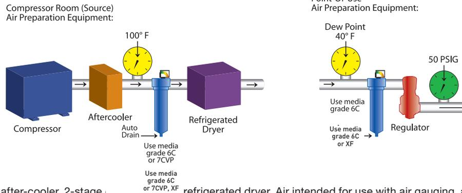
Any compressor with after-cooler, 2-stage refrigerated dryer. Air intended for use with air gauging, air conveyors, spray-painting, food processing, instrumentation, blow molding, cosmetics, film processing, bottling, pharmaceuticals, dairy, breweries, medical, robotics and close tolerance valves.
