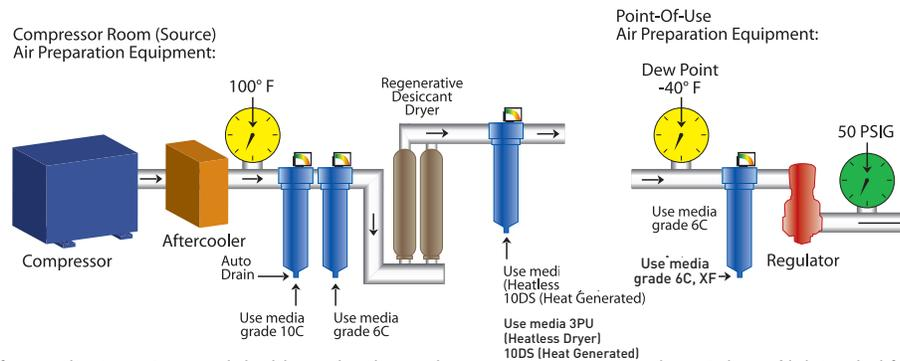
Any compressor with after-cooler, two-stage and double coalescing filter and a regenerative-type desiccant dryer. Air intended for use in applications involving rapid expansion of compressed air, critical instrumentation, high purity gases, computer chip drying, etc.
