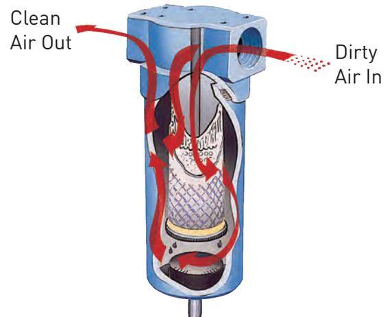
This filter housing cutaway depicts the coalescing process. Air enters the housing and flows through the filter media passing from the inside element surface to the outside. Coalesced liquid collects in the housing where it is drained, and clean air exits the housing through the outlet port.
