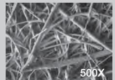
Grade 10 filters are used as prefilters for grade 6 to remove gross amounts of aerosols or tenacious aerosols which are difficult to drain. This grade is often used as a ‘coarse’ coalescer.
