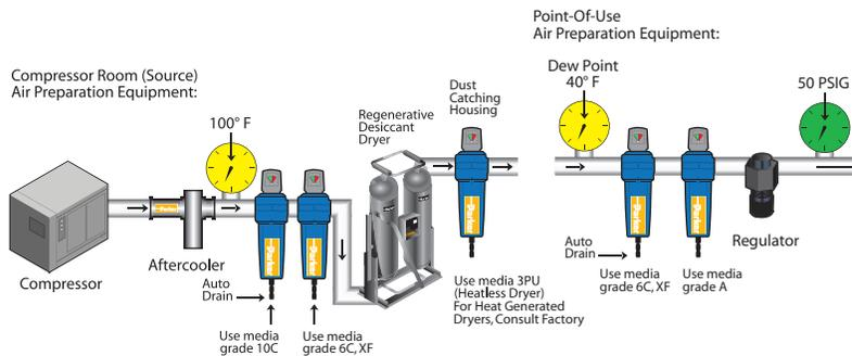
Any compressor with after-cooler, two-stage and double coalescing regenerative-type desiccant dryer and a carbon adsorber. Air intended for use in applications involving rapid expansion of compressed air, critical instrumentation, high purity gases, automotive paint systems, etc. CAUTION: This air is too dry for respiratory use.
