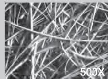
Grade 8 filter elements provide high efficiency filtration in combination with high flow rate and long element life.
