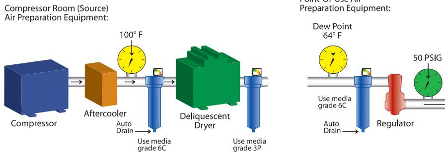
Any compressor with after-cooler, 2-stage coalescing and deliquescent dryer. Air intended for use with general pneumatic systems, body shop spray painting and components sensitive to high moisture content.
