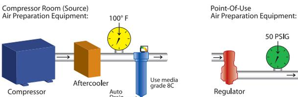
Any compressor with after-cooler. Air intended for use with lubricated air tools, air motors, cylinders, shot blasting, non-frictional valves.
