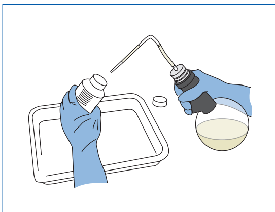
Figure 20. Flushing sample container with solvent filtering dispenser.
