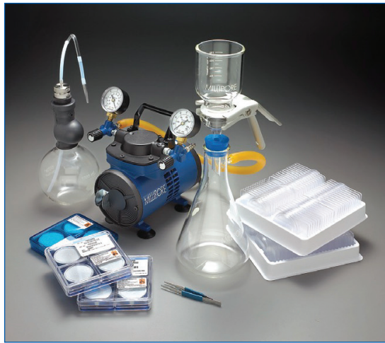
Figure 24. Laboratory Filter Apparatus assembled using the Fluid Contamination Kit (Cat Nos. XX7104711K and XX7104712).
