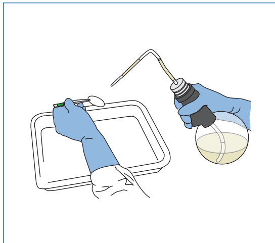
Figure 26. Flushing filter with solvent filtering dispenser.
