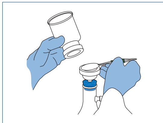
Figure 27. Placing membrane filter on base of 47 mm glass filter holder.
