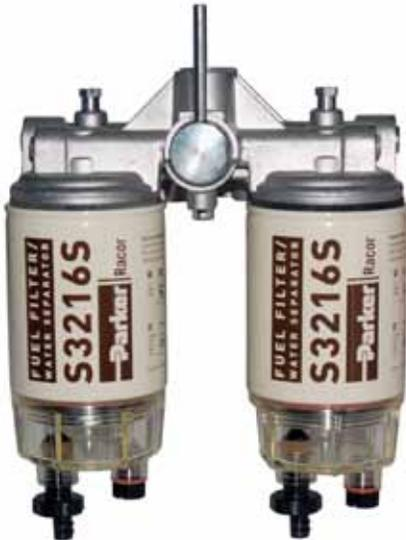
The Racor Dual Spin-On Series provides twice the filtering capacity in one compact and robust package. A shut-off valve located in the mounting head can switch to the clean filter so that the dirty filter may be serviced (servicing filters is not possible while engine is running).
