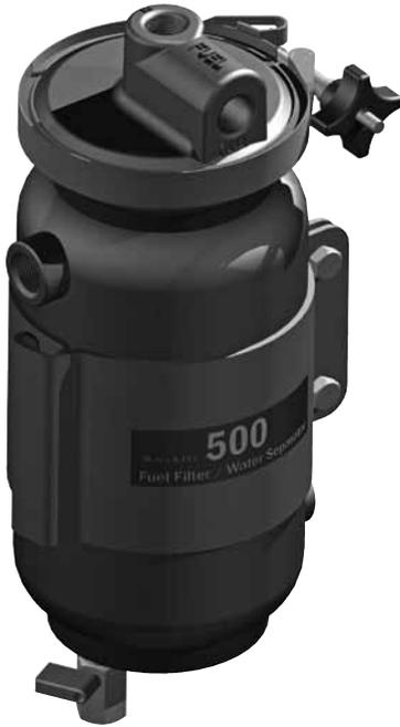
Want proven reliability? A Racor 500 Fuel Heater/Water Separators are for today's high performance heavy-duty and smaller midrange engines. These lightweight aluminum units use engine coolant to produce a 47°F rise in fuel temperature, eliminating the need for fuel blending.
