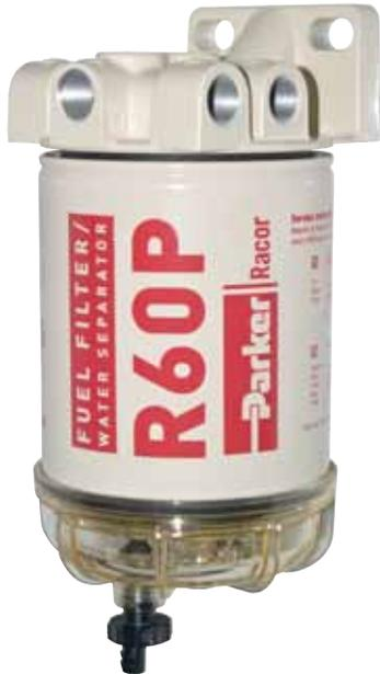
**All 600 Series Spin-On fuel filter/water separators feature multiple fuel ports (4 inlets and 3 outlets) and a unitized mounting bracket for installation convenience. Inlet and outlet threads are 3/8"-18 NPTF for all models. These filter assemblies provide flexibility during mounting and fit any engine application.**
