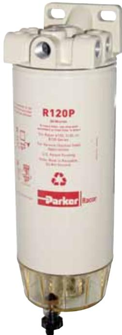
**All 600 Series Spin-On fuel filter/water separators feature multiple fuel ports (4 inlets and 3 outlets) and a unitized mounting bracket for installation convenience. Inlet and outlet threads are 3/8"-18 NPTF for all models. These filter assemblies provide flexibility during mounting and fit any engine application.**
