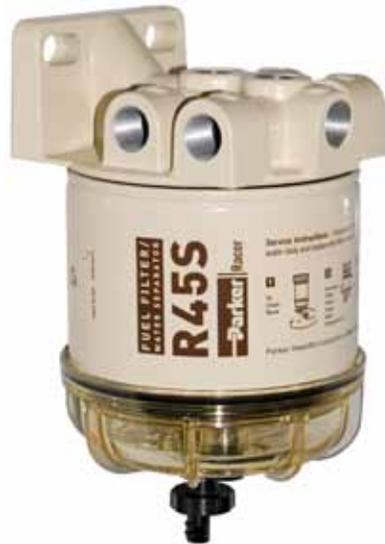
**All 600 Series Spin-On fuel filter/water separators feature multiple fuel ports (4 inlets and 3 outlets) and a unitized mounting bracket for installation convenience. Inlet and outlet threads are 3/8"-18 NPTF for all models. These filter assemblies provide flexibility during mounting and fit any engine application.**
