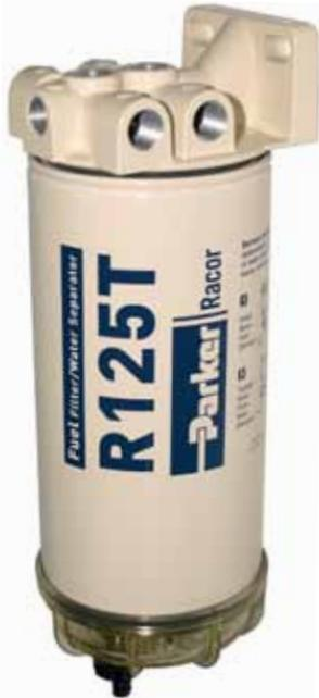
**All 600 Series Spin-On fuel filter/water separators feature multiple fuel ports (4 inlets and 3 outlets) and a unitized mounting bracket for installation convenience. Inlet and outlet threads are 3/8"-18 NPTF for all models. These filter assemblies provide flexibility during mounting and fit any engine application.**
