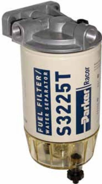
Racor's 325R Diesel Fuel Filter/ Heater/ Water Separators are specifically designed to handle today's tough fuel system problems. These units feature a standard in-head PTC heater and reusable see-thru contaminant collection bowl. They are different only in flow capacity and element size.
