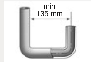
● Minimum clearance of U-shape bends
