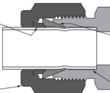
Pressure seal by front ferrule on tube and body
