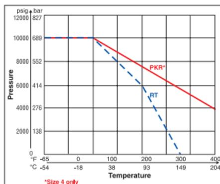
**Note:** This Pressure versus Temperature chart reflects the use of indicated seat materials in Stainless Steel valves without consideration of seal materials.
