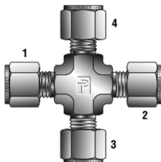
**Type:** A letter or combination of letters and numbers are used to designate the type of fitting. (i.e. SBZ or MBT = male branch tee, GBZ or FA = female adapter, etc.) See the visual index for fitting types.
