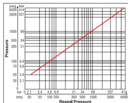
**Note:** Valves which are not actuated for a period of time may initially crack at higher than set crack pressures.
