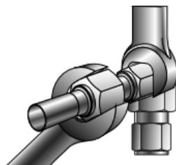
2. Now select the proper size inspection gauge and try to place it, as shown, between the nut and the body hex. If gauge does not fit at any point between them, you have correctly tightened the nut. If you can slip the gauge into the space, the fitting is not properly made up, and you must repeat the assembly procedure.
