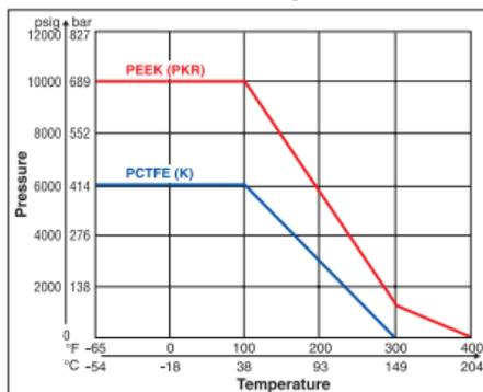
**Note:** This pressure versus temperature chart reflects the maximum temperature range of indicated materials.
